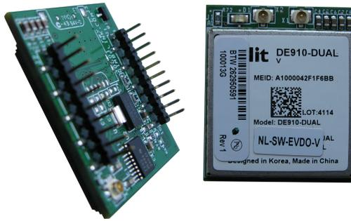
**Figure 5.16:** This is an example of the cellular modem utilized in the communication nodes. The two U.FL connectors allow attachment of antennas for both cellular communication as well as GPS synchronization.
