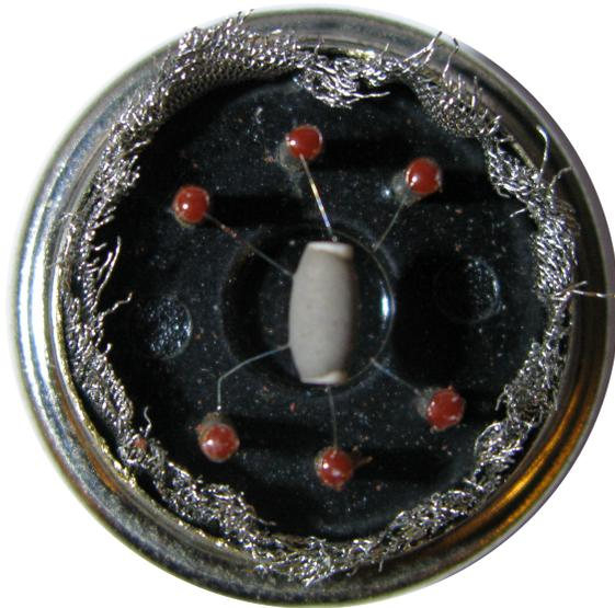
**Figure 5.24:** This image of the MQ-4 sensor with the metal mesh removed shows the actual sensor. A gas sensing layer on an Al<sub>2</sub>O<sub>3</sub> substrate is connected with Au and Pt electrodes. A nichrome filament housed within the ceramic tube heats the area during detection to improve response.
