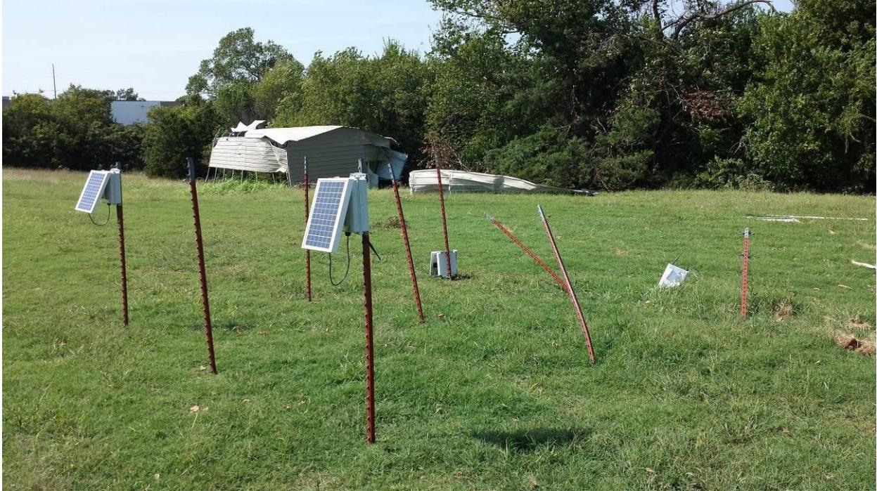
**Figure 6.4:** Severe damage to prototype sensors at test site after debris strike (seen in background) during gusty weather.
