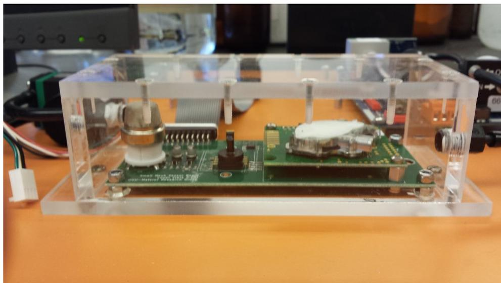
**Figure 5.46:** Lexan box housing sensor board for use in communication nodes. The box has been sealed from external flow by dichloromethane solvent at the joints.
