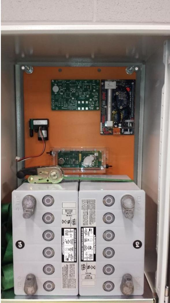
(a) The layout of components within the large communication nodes. The batteries take up most of the space inside the enclosure, so components were arranged to be bolted to the top of the back plate.
